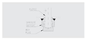
**Step 8**: Screw the compression fitting into the threaded fitting by tightening to 340 Nm torque. Holding the head of the FloTec with a wrench to maintain correct orientation, use a long wrench to tighten the compression fitting until approximately one thread is left exposed under the nut, ensuring the flowmeter does not turn.
