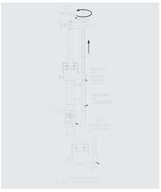
**Step 5**: Once Step 4 is completed, fully close the isolation valve (usually 1.1/2" ball valve type).
