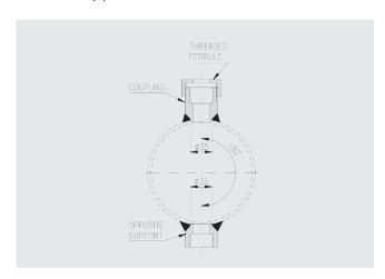
**Step 5**: Repeat steps from 1 to 3 to install the opposite support fitting.
