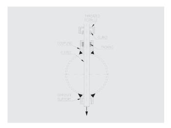
**Step 7**: Insert the FloTec with the threaded ferrule and the gland through the threaded fitting into the pipe and through the opposite support. Apply appropriate sealant and tighten opposite support hex plug. Turn the FloTec until the flow arrow is positioned correctly and the sensor bar tip reaches the bottom of the hex plug.
