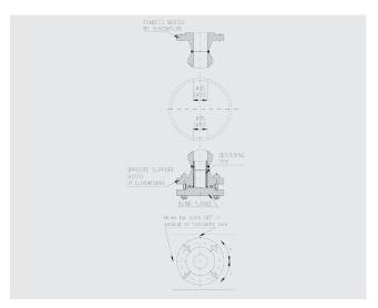
**Step 4**: Insert the FloTec through the nozzle into the pipe and check that the tip protrudes through the hole in the opposite pipe wall when the two flanges mate squarely. Position the end-support cup over the tip of the flowmeter, ensuring the tip is concentric with the hole, and tack-weld the end-support cup in place. Remove the FloTec and complete the support cup weld.
