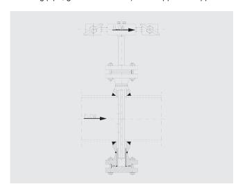
Step 6: Check the FloTec is installed correctly and aligned.
