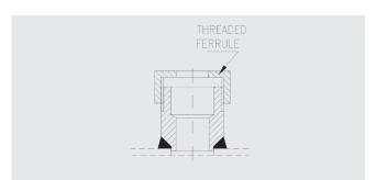
**Step 5**: Insert the FloTec with the threaded ferrule and the gland through the threaded fitting into the pipe. Apply appropriate sealant to the threads of the compression fitting. Turn the FloTec until the flow arrow is positioned correctly and the sensor bar tip reaches the back side of the pipe.
