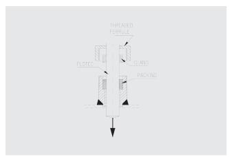
**Step 6**: Screw the compression fitting into the threaded fitting by tightening to 340 Nm torque. Holding the head of the FloTec with a wrench to maintain correct orientation, use a long wrench to tighten the compression fitting until approximately one thread is left exposed under the nut, ensuring the flowmeter does not turn.
