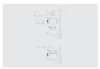
**Step 4**: Turn the handwheel till the green band painted on the threaded rod reaches its end limit (extracted position).
