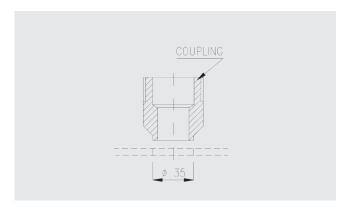
**Step 2**: Align the threaded fitting concentrically over the hole and tack-weld in place. Using a suitably sized and threaded length of pipe, check the threaded fitting is concentric and aligned correctly.
