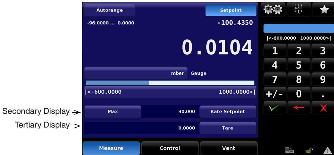
Figure 6.2.9a - Secondary and Tertiary Displays
