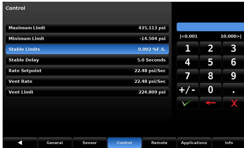
Figure 7.3.2a - Stable Limits and Stable Delay
