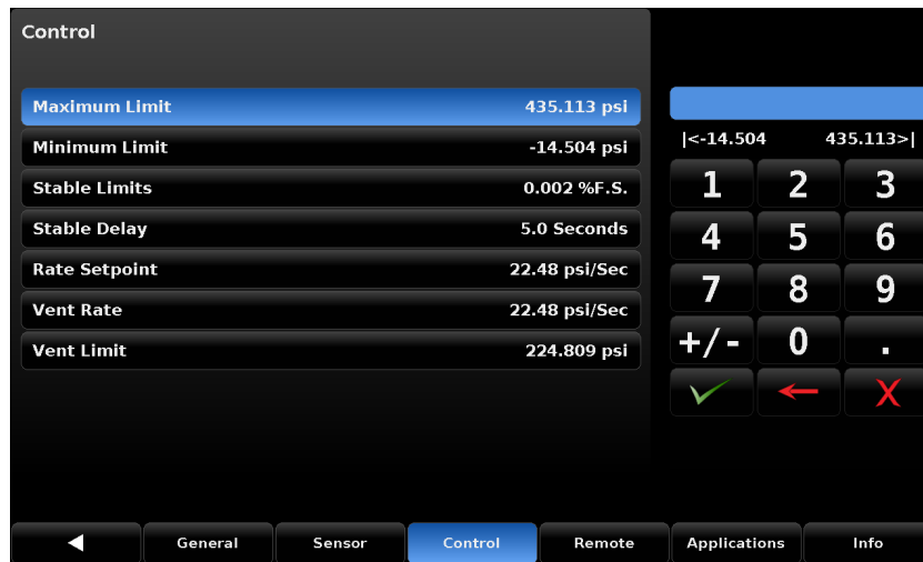
Figure 7.3.1 - Maximum Limit and Minimum Limit Buttons
