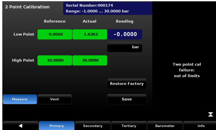
Figure 7.5.2.5.2-9 – ‘2 Point Calibration Failure’
