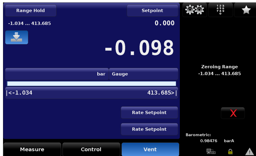
Figure 6.2.14-A Zero Button in Gauge
