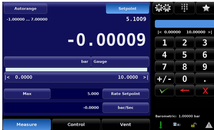
Figure 6.2.4 - Output Pressure Setpoint
